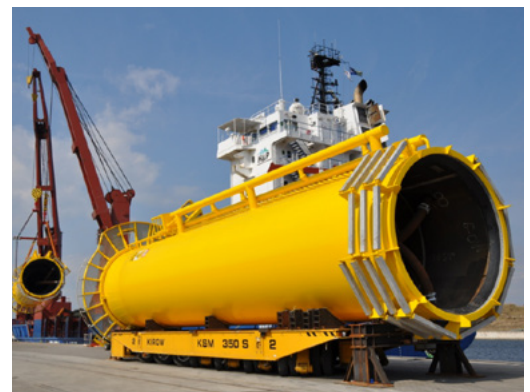
Transition Pieces for Walney Windfarm
