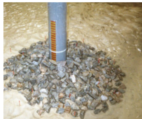
Model test with Monopile foundation at movable seabed. Situation after sand bank has been eroded.
