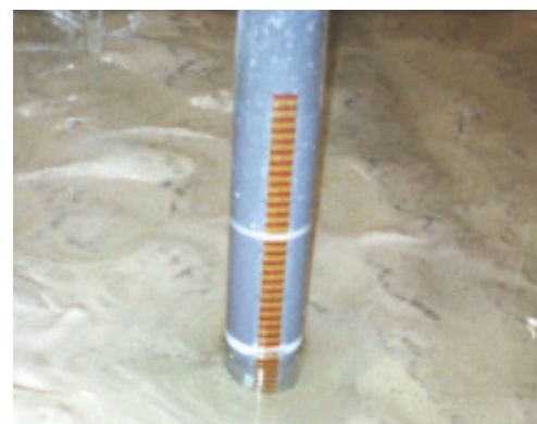
Scour around a circular cylinder during combined waves and current. Notice the relative limited scour development due to the presence of waves.
