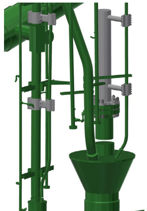
Laser scan model, basis for detailed geometrical design of reinforcement clamps
