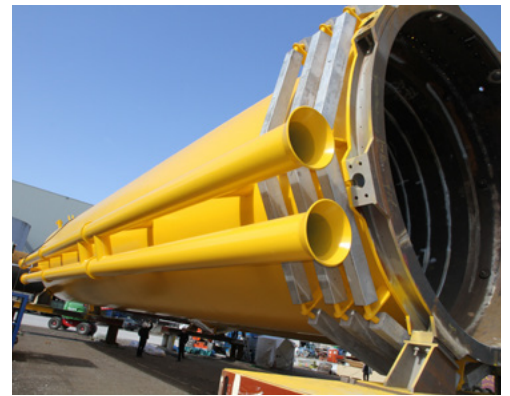
Monopile for Northwind, ready for installation
