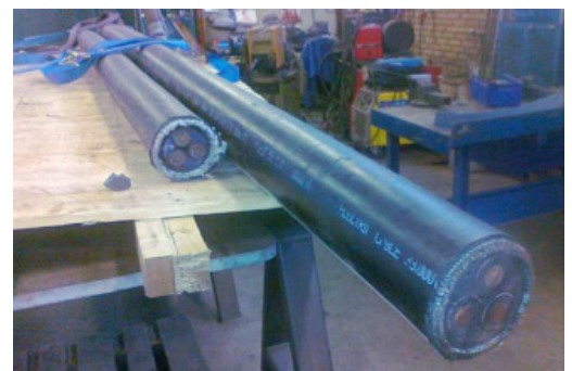
Typical Array Cables
