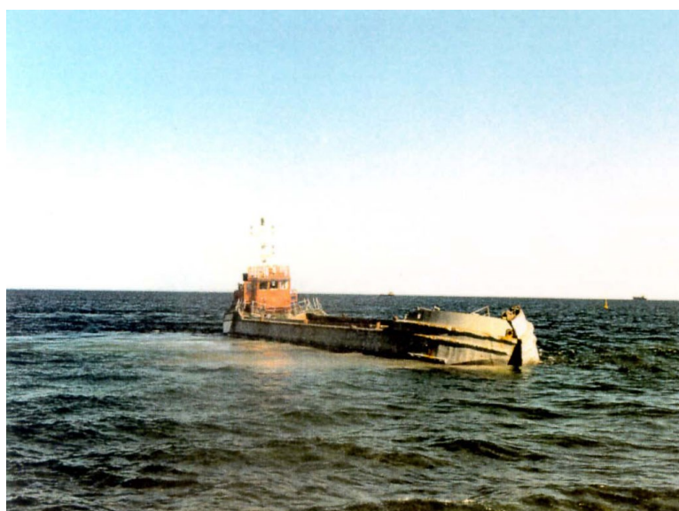
Depositing of material from split barge
